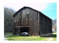
parent reason for that shape. This barn is sided with vertical boards in such a manner as to provide long, tall vent doors of one or two boards wide on metal hinges, to be opened as needed for increased air flow for the air curing of the tobacco. This farm sits in the Big Creek valley and was part of the Gaither Shelton farm.
